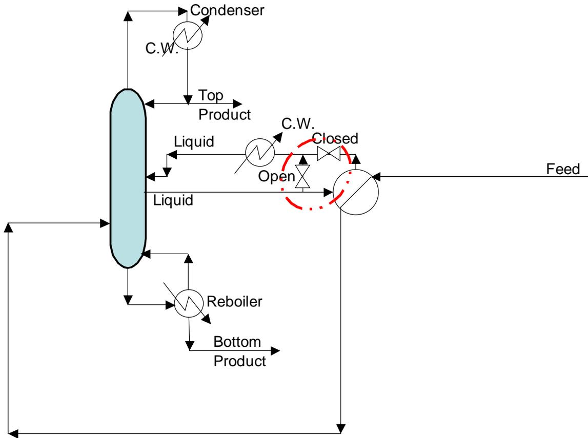
Figure 3: Unnecessary Bypassing of Heat Recovery Equipment
