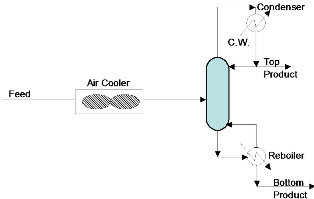
Figure 1: Inappropriate Cooling of Distillation Column Feed
