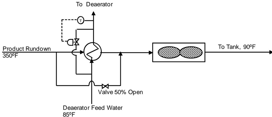
**Figure 10:** Deaerator Feed Water Preheat Project, with Manual Bypass on Product Rundown
