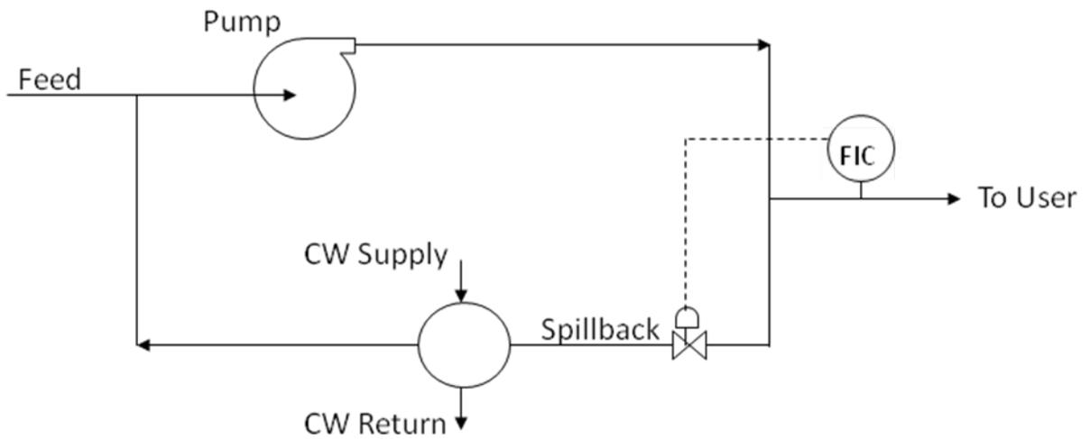
Figure 5: High Pressure Feed Pump with Spillback Control
