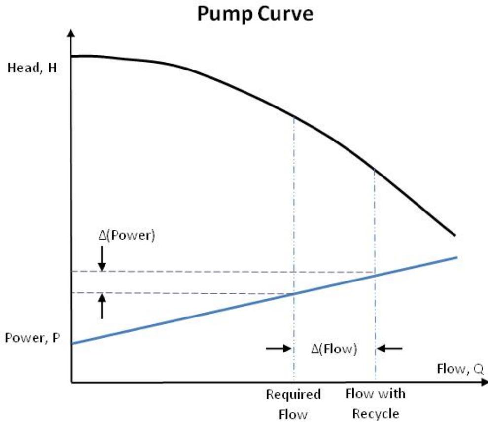
Figure 6: Pump Curve Comparing Spillback and Throttle Control
