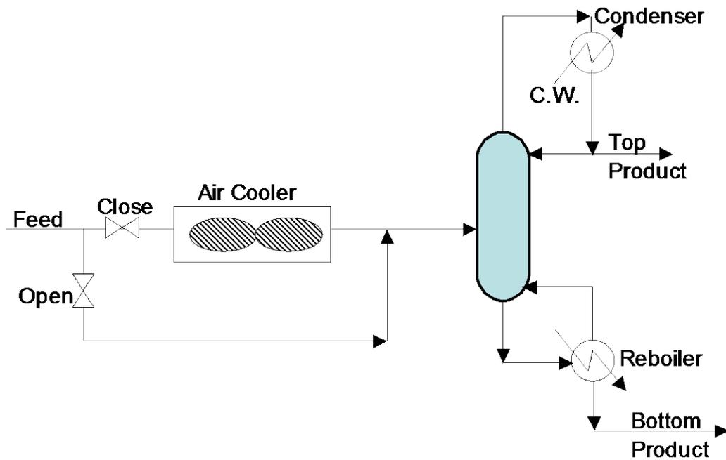
**Figure 2:** Inappropriate Cooling Corrected by Bypassing Cooler on Distillation Column Feed
