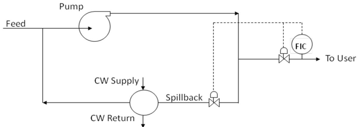
Figure 7: High Pressure Feed Pump with Throttle Control
