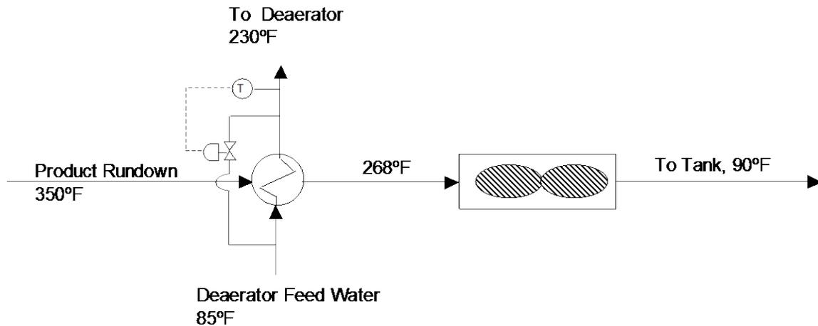
Figure 9: Deaerator Feed Water Preheat Project, as Originally Implemented
