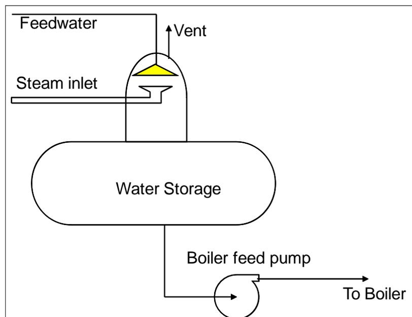
Figure 8: Thermal Deaerator – Main Components
