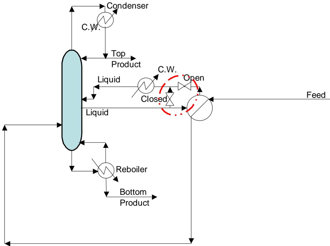
**Figure 4:** Closing the Bypass Restores Heat Recovery
