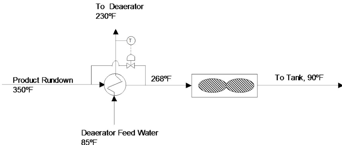
**Figure 11:** Deaerator Feed Water Preheat Project, with Automatic Temperature Control on Product Rundown Bypass
