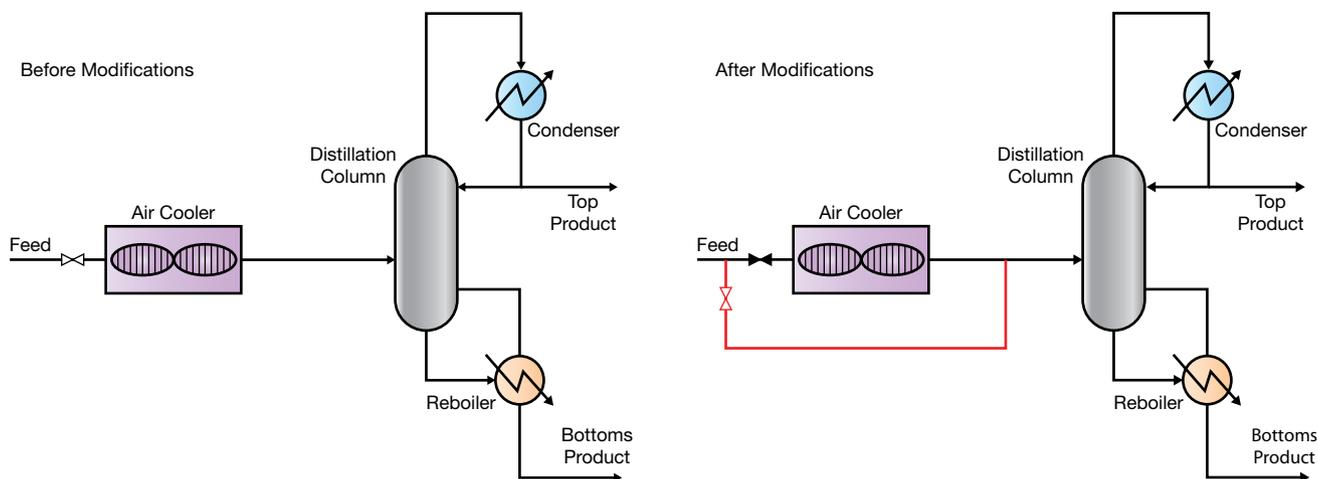
▲ **Figure 3.** This distillation system includes an air cooler that was designed to run only during abnormal conditions, but was run continuously instead. Identifying this equipment misuse and turning off the air cooler saved energy. Even after the operational change, additional heat was still being lost to convection in the cooler, so a bypass was installed (right, red).
