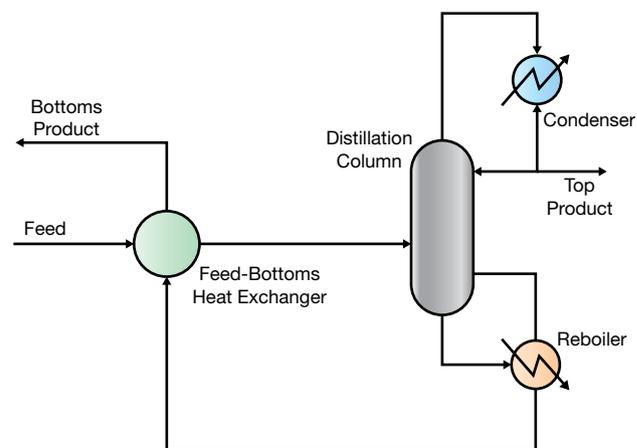
▲ **Figure 2.** This distillation column system includes a feed-bottoms heat exchanger (FBHE) at the inlet to heat the feed with the hot bottoms stream. Although this reduces the energy requirements for the reboiler, the heated feed has the potential to increase vapor traffic above the feed tray of the distillation column, which may overload the condenser.
