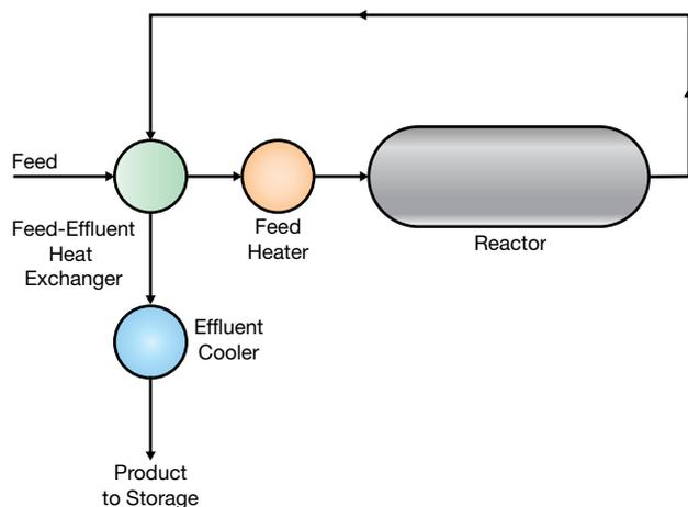
▲ **Figure 1.** The feed-effluent heat exchanger (FEHE) uses the hot effluent stream from the reactor to heat the cold incoming feed. The incoming feed also cools the product stream before it is sent to storage. By pairing streams, the energy requirements of the effluent cooler and feed heater are both reduced.
