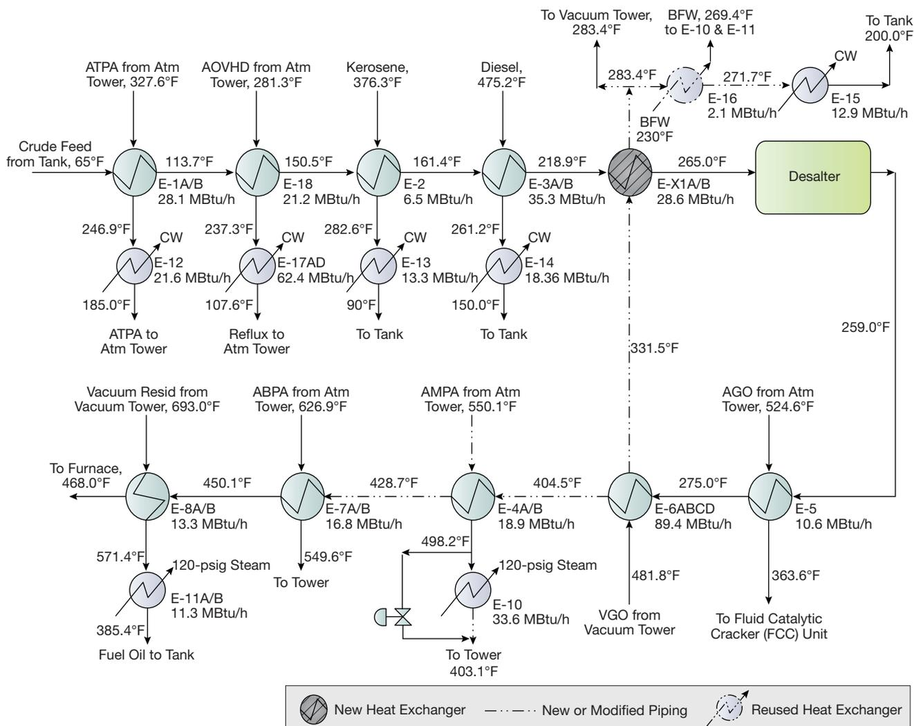
▲ **Figure 6.** The final design requires just one new pair of heat exchanger shells and repiping of some existing equipment.
