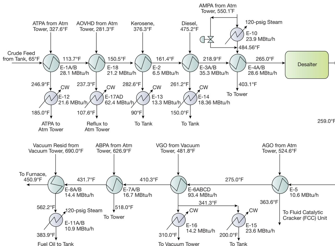
▲ **Figure 3.** Heat from the pumparounds, product rundowns, and atmospheric tower overheads is recovered in the existing crude preheat train. Excess heat is removed in steam generation and cooling water.
