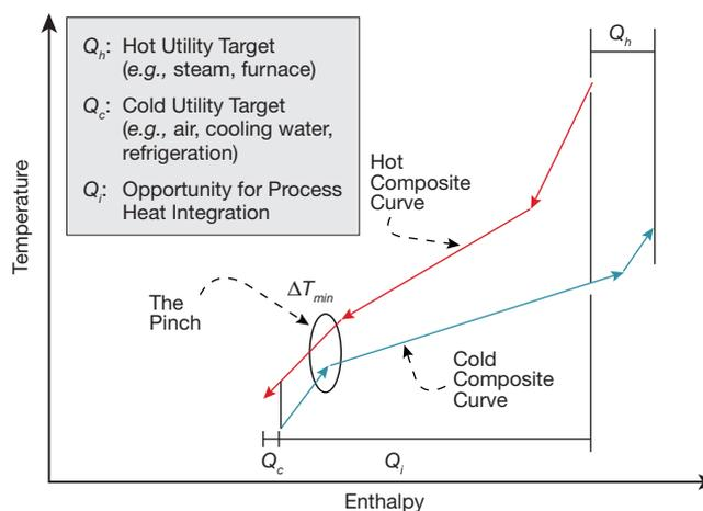
▲ **Figure 1.** Composite curves show the combined heat sources and combined heat sinks in any process as temperature vs. enthalpy plots. The curves can be used to determine how much heat can be recovered by heat integration and how much has to be supplied or removed by external utilities.
