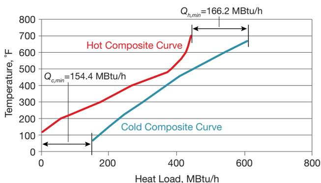
▲ Figure 4. The composite curves for the crude unit example show the combined heat sources and combined heat sinks as temperature vs. enthalpy plots.
