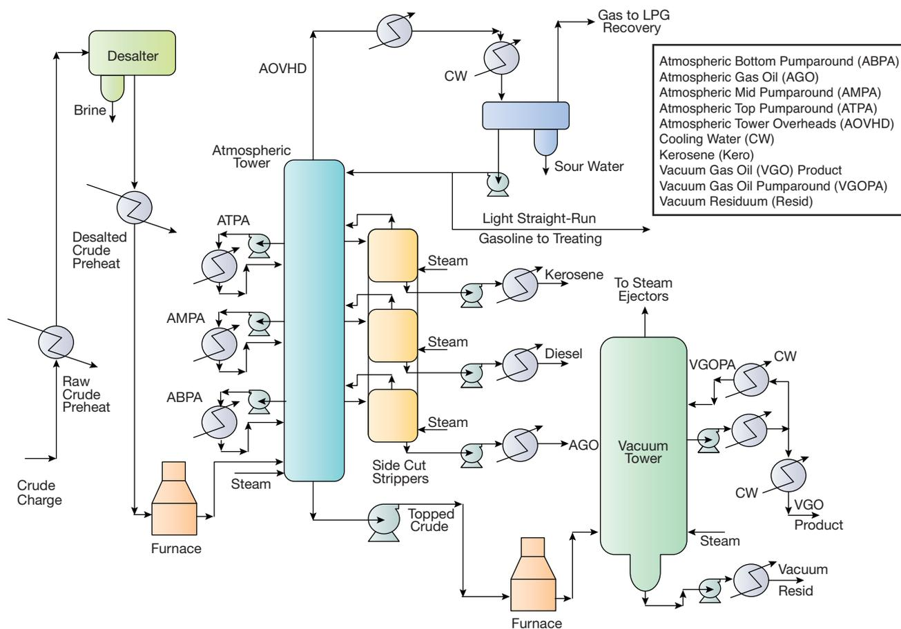
▲ **Figure 2.** The crude distillation unit uses both an atmospheric tower and a vacuum tower to fractionate crude oil. Pumparounds are used to control cut points and remove heat at the highest practical temperature levels.
