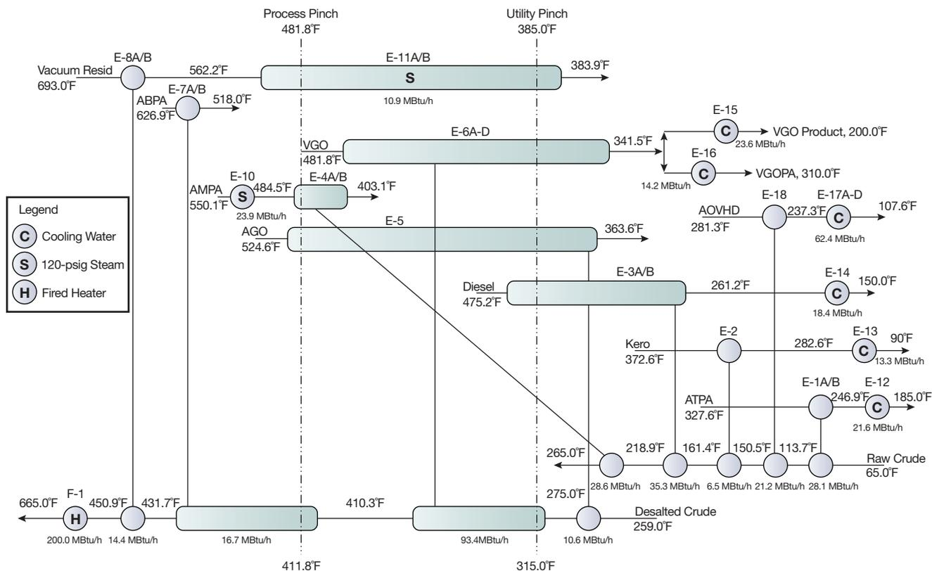
▲ Figure 5. Representing the existing preheat train as a grid diagram highlights inefficient cross-pinch heat exchangers.
