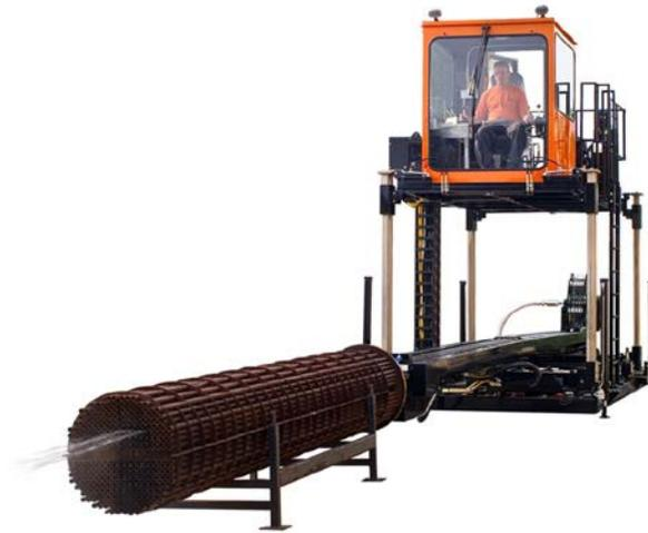
**Figure 1: Shell-side (left) and Tube-side (right) Hydroblasting Equipment for Cleaning Shell & Tube Heat Exchangers. Photos courtesy of NLB Corporation.**
